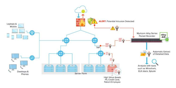
Figure 1: Myricom nVoy AIR watching critical assets and ready to respond to intrusion events.
